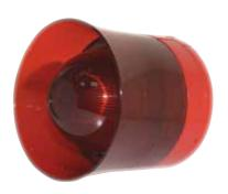
When individual address reporting is not required, NGA-504 ASB can be configured as a Shadow sounder. In this case sounders do not occupy and address i nthe loop thus freeing up addresses for more detection devices. Shadow sounders do not report back to the control panel so their presence on the loop is not monitored. Shadow sounders draw current from the loop (10mA in alarm) and must be included in loop load calculations.
