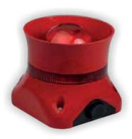
When individual address reporting is not required, NGA-504 AS WP can be configured as a shadow sounder. In this case sounders do not occupy an address in the loop thus freeing up addresses for more detection devices. Shadow sounders do not report back to the control panel so their presence on the loop is not monitored. Shadow sounders draw current from loop (10mA in alarm) and must be included in loop load calculation.
