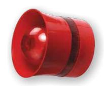
When individual address reporting is not required, NGA-504 AS can be configured as a shadow sounder. In this case sounders do not occupy an address in the loop thus freeing up addresses for more detection devices. Shadow sounders do not report back to the control panel so their presence on the loop is not monitored. Shadow sounders draw current from loop (10mA in alarm) and must be included in loop load calculation.
