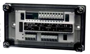
The connection to each NGA-700 is monitored for fault (open or short-circuit) and Alarm conditions. The interface is used to monitor the contacts of an external system which must be interfaced to the Fire Alarm system, for example a Flow switch in a sprinkler system to indicate if the sprinklers have been activated or extinguishant level monitoring in Gas Extinguishing System, etc.
