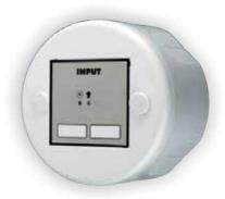
The connection to the NGA-700 is monitored for Fault (open or short circuit) and Alarm conditions. The interface is used to monitor the contacts of an external system which must be interfaced to the Fire Alarm System, for example a flow switch in a sprinkler system to indicate if the sprinkler have been activated or extinguish and level monitoring in GAs Extinguishing systems etc.
