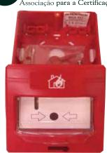
A bi-colour LED flashes Green when the unit is interrogated by the control panel and is illuminate Red when in alarm. The command to illuminate the Red LED is emitted by the control panel in response to activation of the individual call point thus confirming that the alarm signal has been received at control panel.
